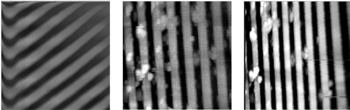
(a) 三角波驱动方式的扫描图 (b) 正弦波驱动方式的扫描图 (c) 正弦波驱动方式的有畸变的扫描图 (a) Image by triangle signal (b) Image by sinusoidal signal (c) Distorting image by sinusoidal signal
